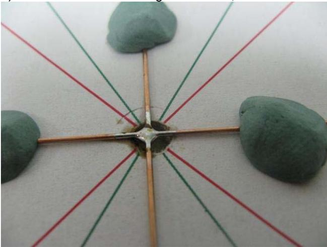
9) Flux the tip of "D", heat your "blob" and install it in the center. Try not do make it stick the other side of the "blob". It must stand vertical.
