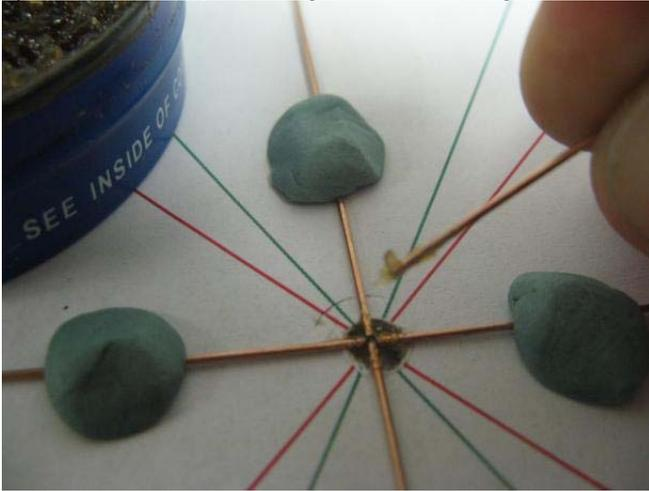
8) Solder the center forming a nice blob, solder must creep on the wires.
