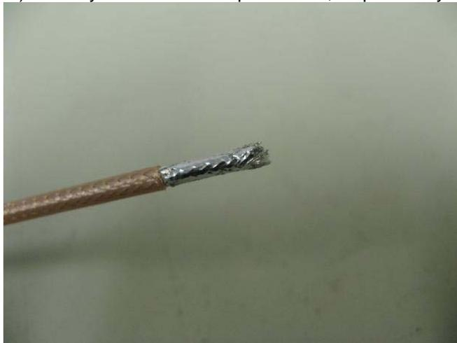
13) Score the tinned coax all around at 3/16" from the tip with the Xacto blade
