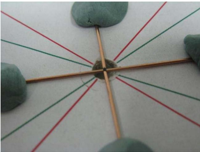
7) Flux the center, don't rely on core-flux in your solder wire, **USE FLUX**.
