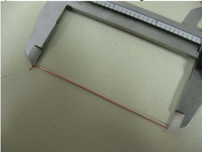
5) Measure one piece of "D" length (cut it a bit longer), file it down to just the right length.
