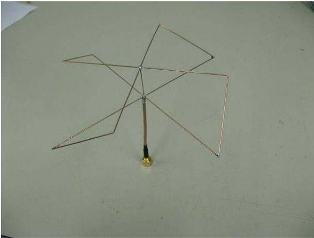
If you build this antenna with a 0.001" caliper, respecting all steps, you'll be within a 1% window of your target frequency. No need for a network analyzer. The nice thing about this antenna is that the higher the frequency, the larger the bandwidth, so tolerances don't grow thinner with 2.4 and 5.8ghz.
