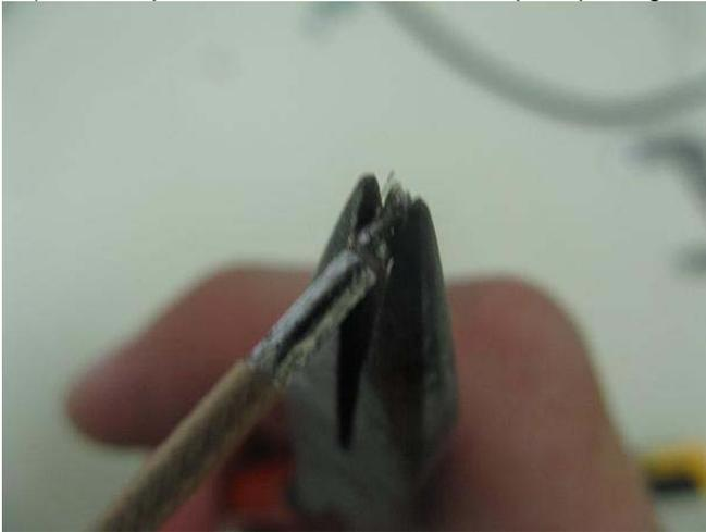
15) Strip around 1/8" of coax center and tin the exposed conductor.
