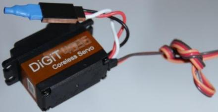
The dummy pots plug into the servo motors NOT the wiring harness.
