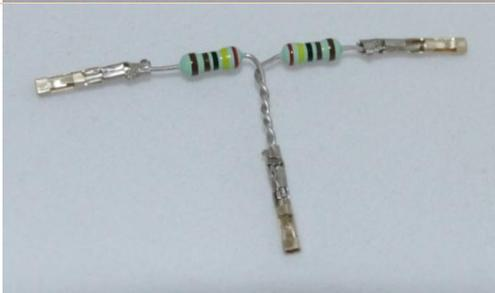
Use pliers to crimp the pins onto the ends of the resistors. It is easier to work with the ends if you separate them from each other
