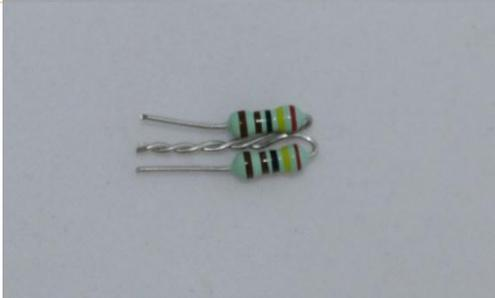
Fold the resistors leads together and the three ends to the same length with at least 1cm to spare.
