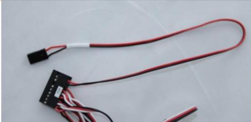
Plug the red wire “roll pot” pin into the skyline connector in the second position from the right on the top row.
