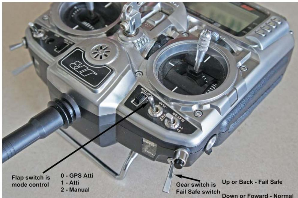
2. Setup a new airplane ACRO model in the transmitter. Give it a name and select a number in the model sequence. If you've forgotten how to do this, just check the manual. If you've lost the manual, download one from the JR web site.
