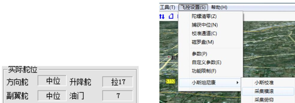
Second, lean the frame to left around 10~15°, then observe the actual servo value in GCS and the gimbal attitude. If the gimbal can get vertical automatically, then same as the first step, observe the value of **【aileron】** under actual servo(must be controlled around 35, not beyond 40), then click on
